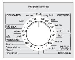
■ Turn the program selector in either direction to the desired program.
